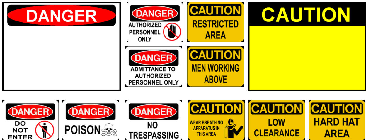
Figure 26: Examples of the Danger and Caution signs used according to Subpart G
